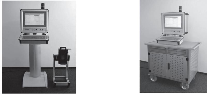
Fig. 10. UER and UER-T system (IZFP, Version 2013) to evaluate the stress state of the rim of railroad wheels
