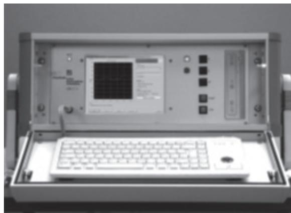
Fig. 7. UER and UER-T systems to evaluate the stress state of the rims of railroad wheels
