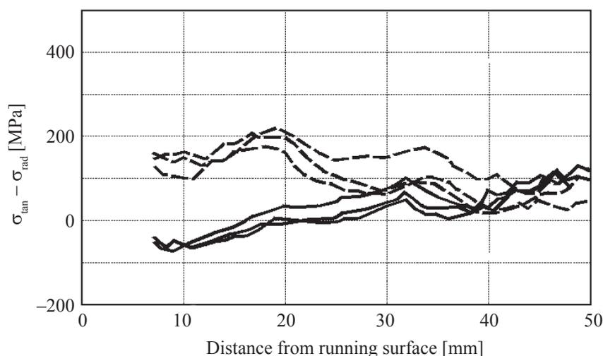
Fig. 5. Result of the ultrasonic stress analysis on new wheels before and after (dotted line) the application of a braking program as used during the downhill passage of the south ramp from the alps
