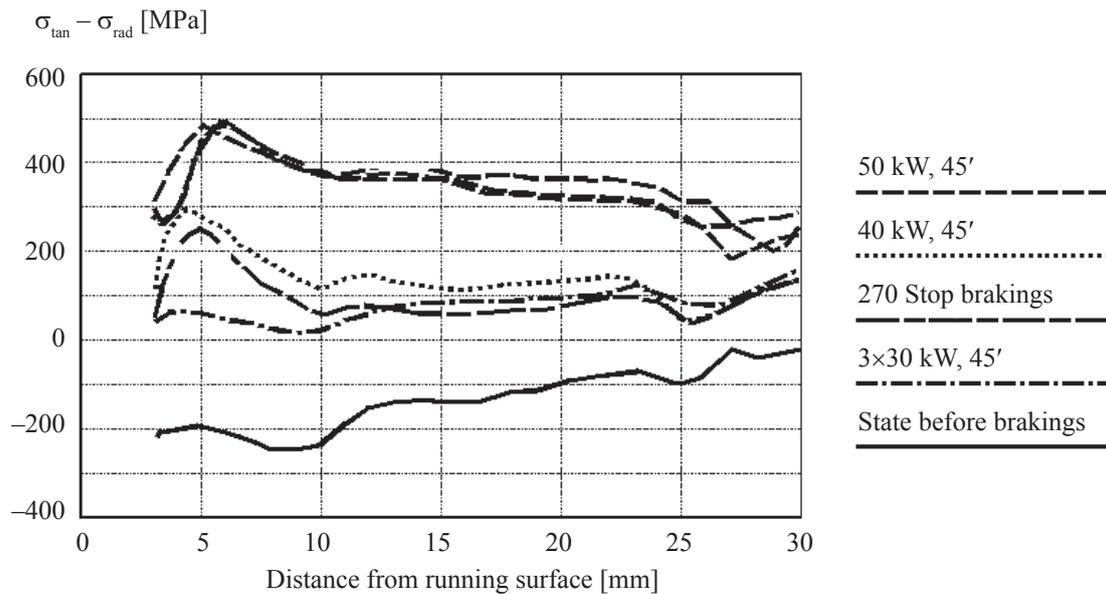
Fig. 4. Change of stress state of the rim of a new wheel after different brakings
