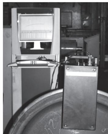
Fig. 9. УКОН-01 system to evaluate the stress state of the rims of wheels
