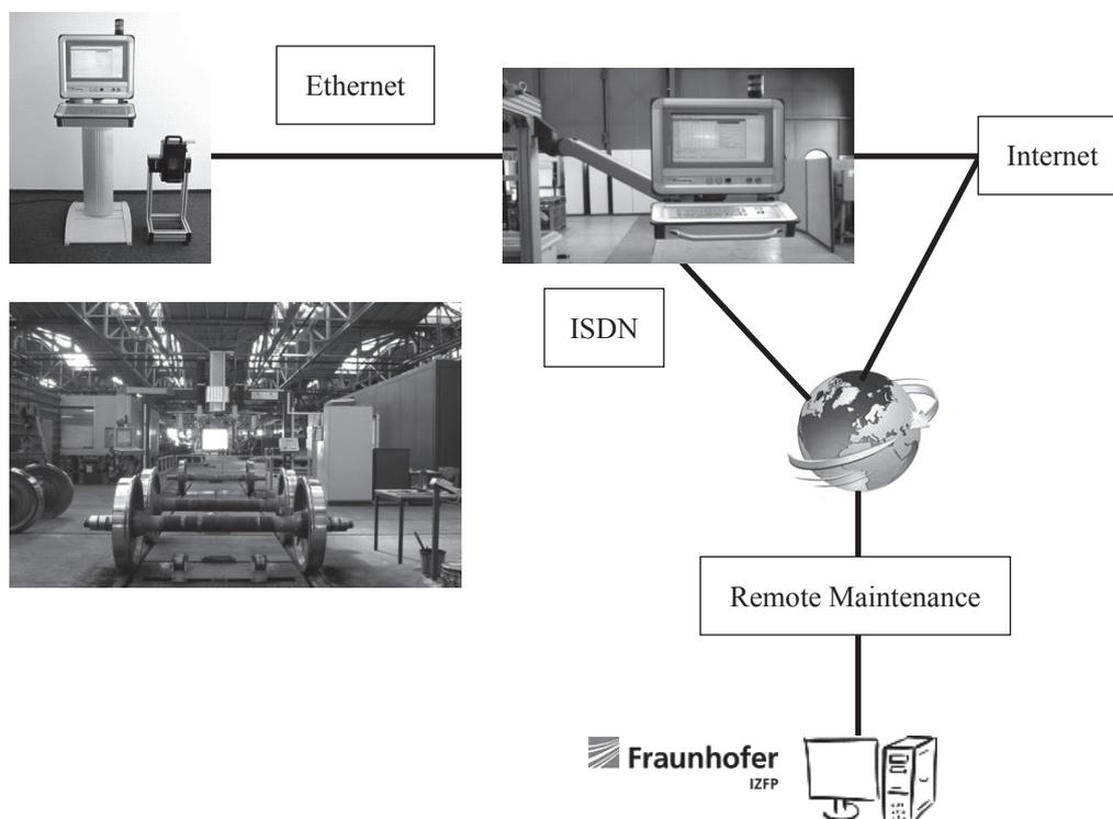
Fig. 11. Sketch of the remote maintenance feature of the UER, UER-T systems
