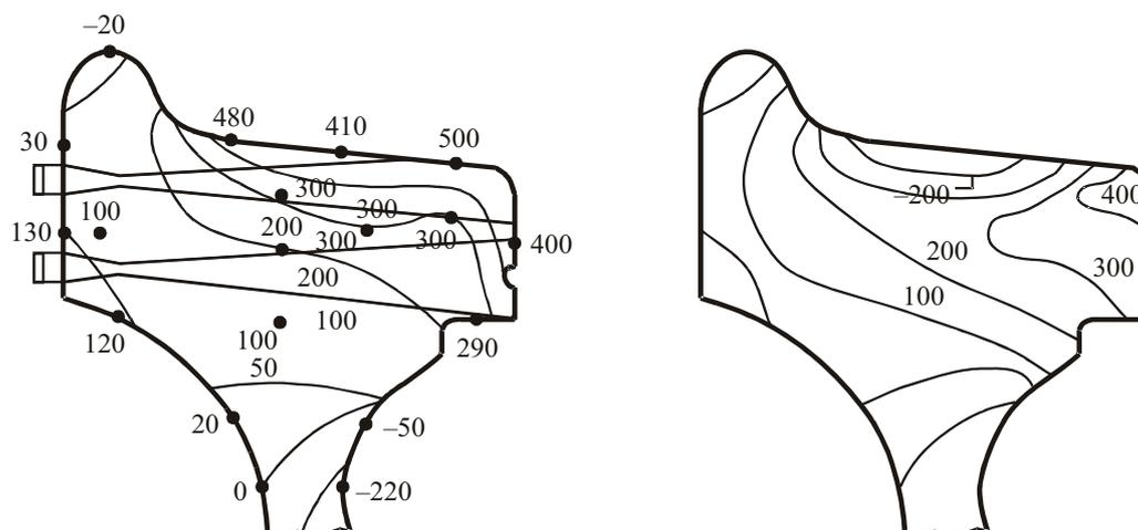
Fig. 1. Distribution of the circumferential stress state [MPa] of a used (left part) and of a new (right part) monoblock wheel
