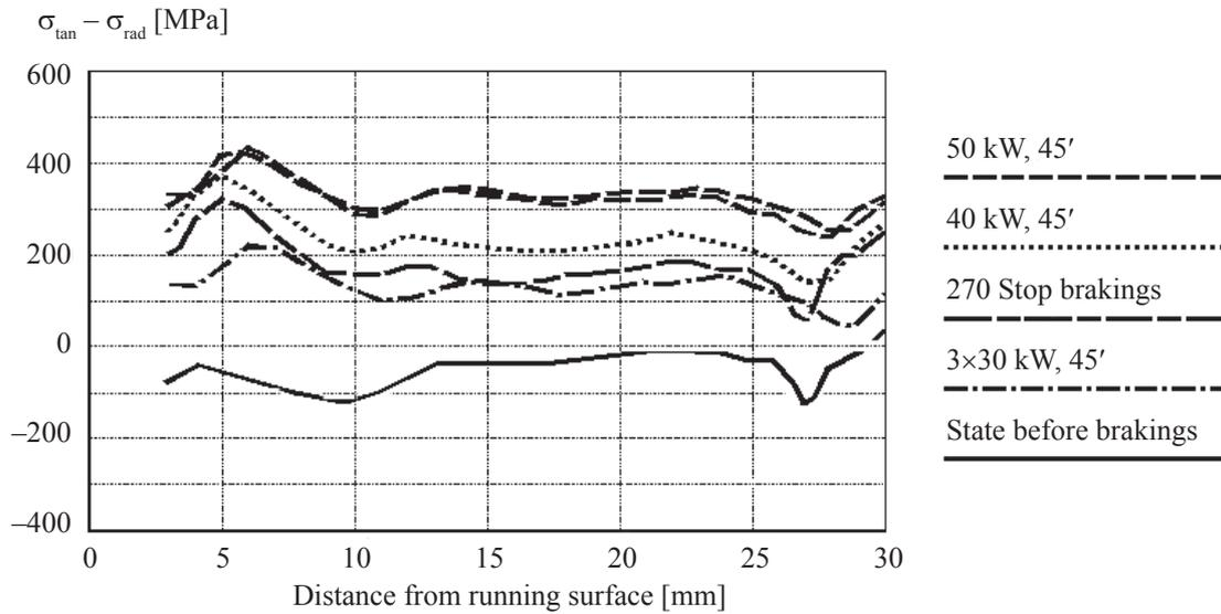
Fig. 3. Change of stress state of the rim of a new wheel after different brakings
