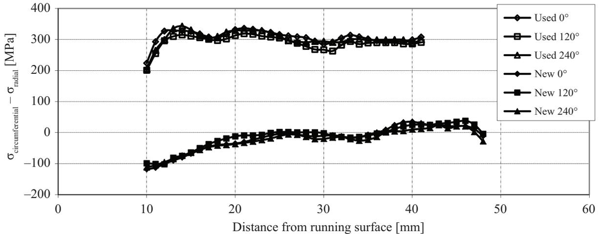
Fig. 6. Stress-depth-profiles of a new and an used wheel evaluated at different positions along the circumference of the wheel
