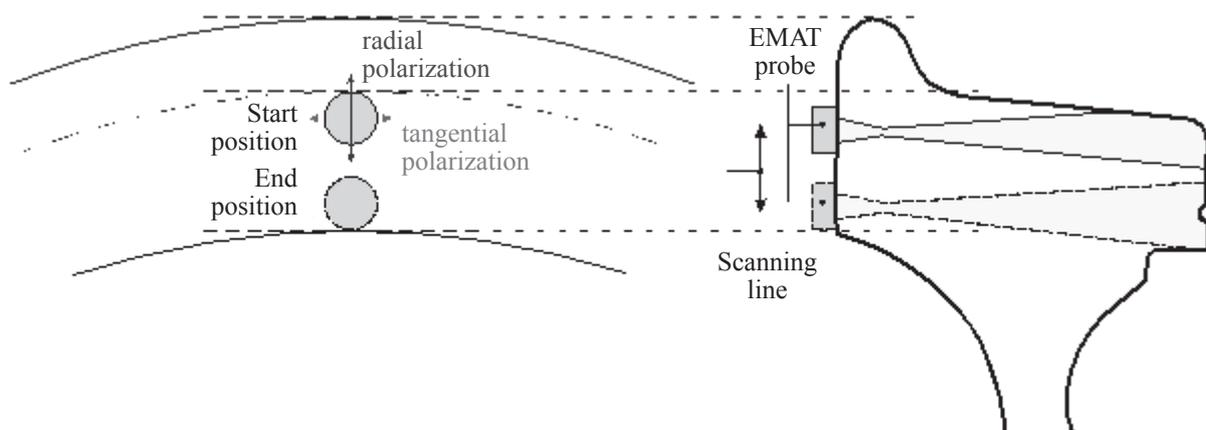
Fig. 2. Sketch of the measuring principle of the ultrasonic technique to evaluate the stress state of railroad monoblock wheels
